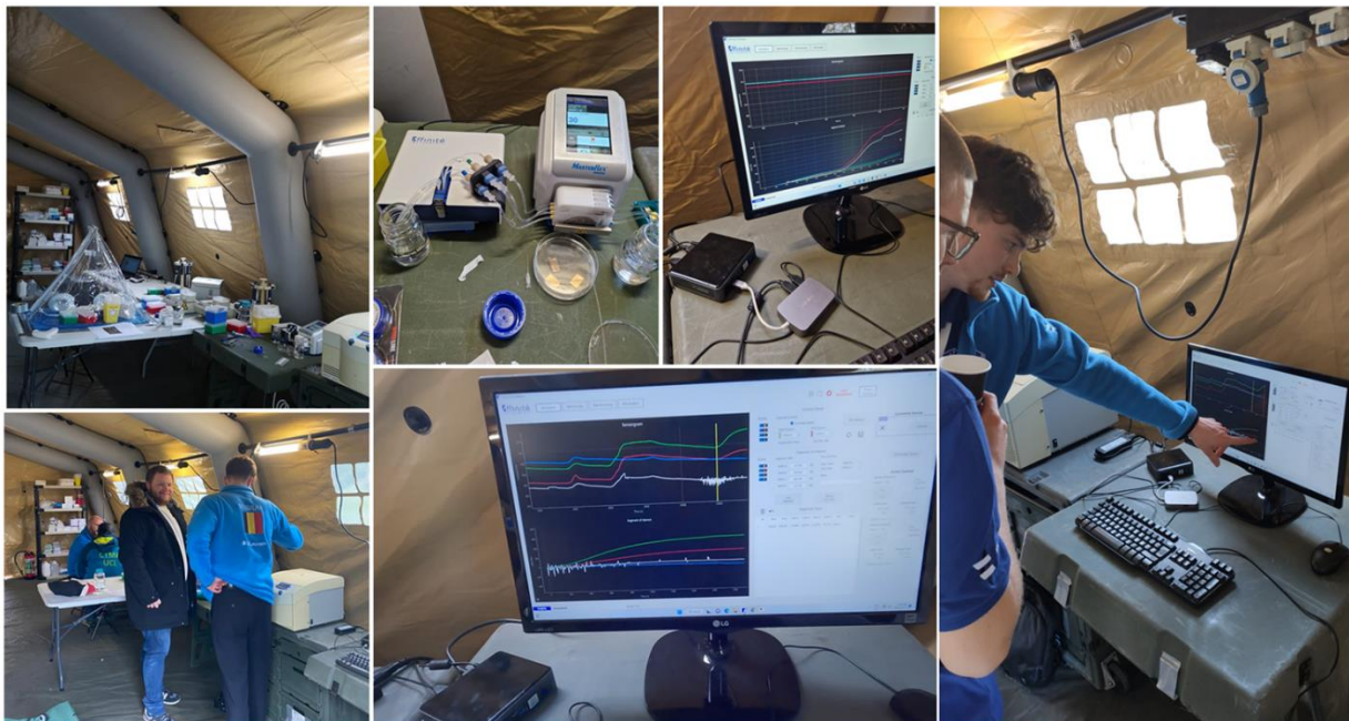
Figure 12. Camelid antibody-based SPR detection of ricin conducted by B-LiFE in the field (eNOTICE, Ranst, 13 May 2023)
